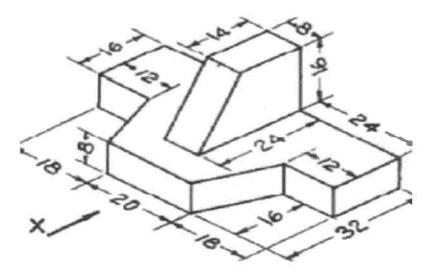
**Q.5(B)** Draw the isometric view of the object, the multi view projection of which 12M 5 4 is shown below:
